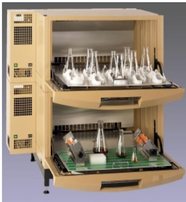
With a modest cabinet footprint the MULTITRON II platform (850 x 470mm) accepts large numbers of Erlenmeyer flasks. The Universal and dedicated platforms are designed with threaded holes for mounting of INFORS clamps and test tube racks. The slide-out shelf option allows the Multitron II to double as a static incubator. The shelf is easy to load and is also removable. When installed, the slide-out shelf limits the flask height to 12".
