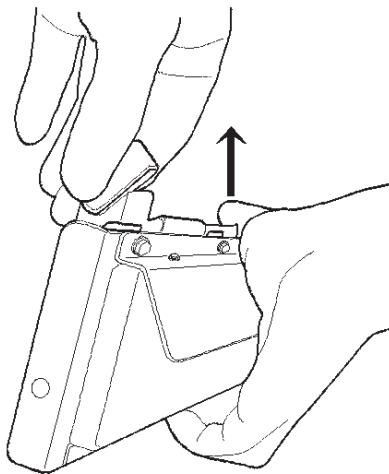
7 Before installing the new Epi light, ensure that the latch is sprung open (upwards).
