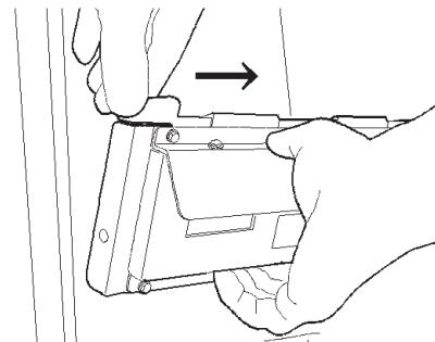
10 Lower the latch to lock the Epi light in place.
