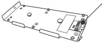
Figure 2.1: Incident (Epi) light source connector (rear)
