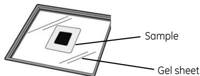
**Note:** *The gel sheet can be used repeatedly. After use, wash it with mild detergent, rinse with water then dry well. A gel sheet can be reused about 20 times.*
