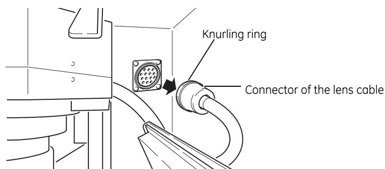
**Note:** Be sure to connect the lens cable. Otherwise, the high sensitivity lens cannot be recognized. This may cause malfunction of the equipment.
