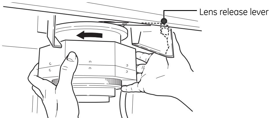
8 Rotate the lens to the left by 45 degrees.
