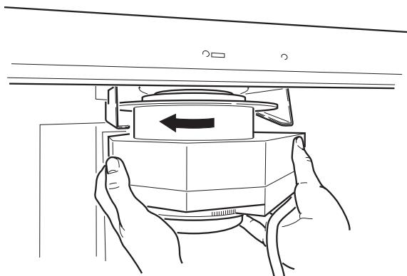
**Note:** Hold the lens with both hands so as to prevent the lens guide from being damaged.
