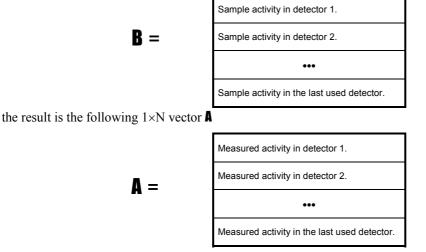
Thus  $\mathbf{A} = \mathbf{MB}$ . Then the matrix  $\mathbf{M}$  is inverted. Let us denote the inverted matrix with  $\mathbf{M}^{-1}$ . When this is multiplied during assay counting with a vector consisting of the measured CPM values in all used detectors, the result vector consists of crosstalk corrected sample activities in those detectors, that is  $\mathbf{B} = \mathbf{M}^{-1}\mathbf{A}$ .
