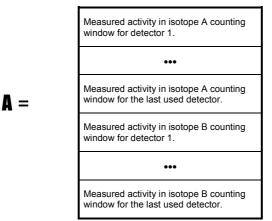
Thus  $\mathbf{A} = \mathbf{MB}$ . Then the matrix  $\mathbf{M}$  is inverted. Let us denote the inverted matrix with  $\mathbf{M}^{-1}$ . When this is multiplied during assay counting with a vector consisting of the measured CPM values in both counting windows and for all detectors, the result vector consists of spillover and crosstalk corrected isotope activities for all detectors, that is  $\mathbf{B} = \mathbf{M}^{-1}\mathbf{A}$ .
