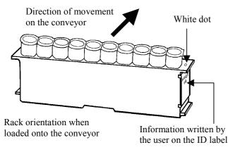
The handwritten information on the label at the end of the rack is then clearly visible from the side of the conveyor.
