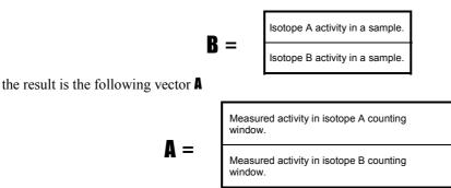
Thus  $\mathbf{A} = \mathbf{MB}$ . Then for each detector the matrix  $\mathbf{M}$  is inverted. Let us denote the inverted matrix with  $\mathbf{M}^{-1}$ . When this is multiplied during assay counting with a vector consisting of the measured CPM values in both counting windows, the resulting vector consists of spillover corrected isotope activities, that is  $\mathbf{B} = \mathbf{M}^{-1}\mathbf{A}$
