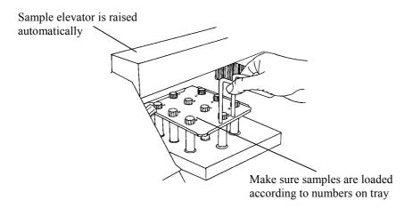
Note: the change to manual mode cannot happen while the cover over the detector block is open. This is because the change to manual mode causes the raising of the arm which transports samples from the conveyor to the detector block to make space for the sample tray to be loaded. For safety reasons this movement cannot happen without the cover being closed. Afterwards the cover must be opened for accessing the detector block.
