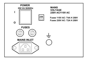
The mains selector in older instruments has the voltage marked on it and is combined with the fuse carriers. To adjust the mains selector, pull it out, turn it through 180 degrees and replace it.
