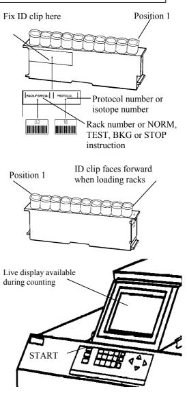
The built-in program allows counting and normalization protocols to be created and edited. The built-in display and keyboard is used. Results are sent to the display and a printer.
