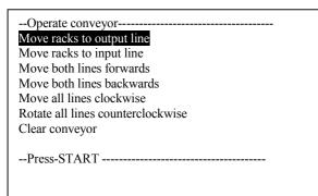
By selecting from this menu and pressing E you can control the movement of racks on the conveyor. To return to the main display, press EXIT.
