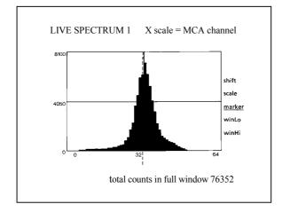
On the right hand side of the spectrum five functions are displayed. By using the up and down arrow keys you can select the function you want. A function is shown to be selected by the underline mark appearing under the function name. The functions are as follows:
