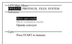
4. Check the time and date by selecting SYSTEM mode and DATE. If it is not correct then give the correct value (See "System | Time & Date setting"). Return to the main display by pressing EXIT.
