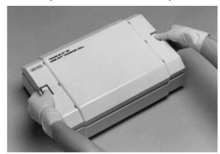
1. Remove the safety cover and the stainless steel cathode assembly.
