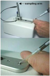
1. With the sampling arm open, pipette the sample onto the lower measurement pedestal.
