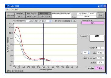
The default option is set to clear the display for the next reading. The user may set the overlay control to clear after each sample plot
